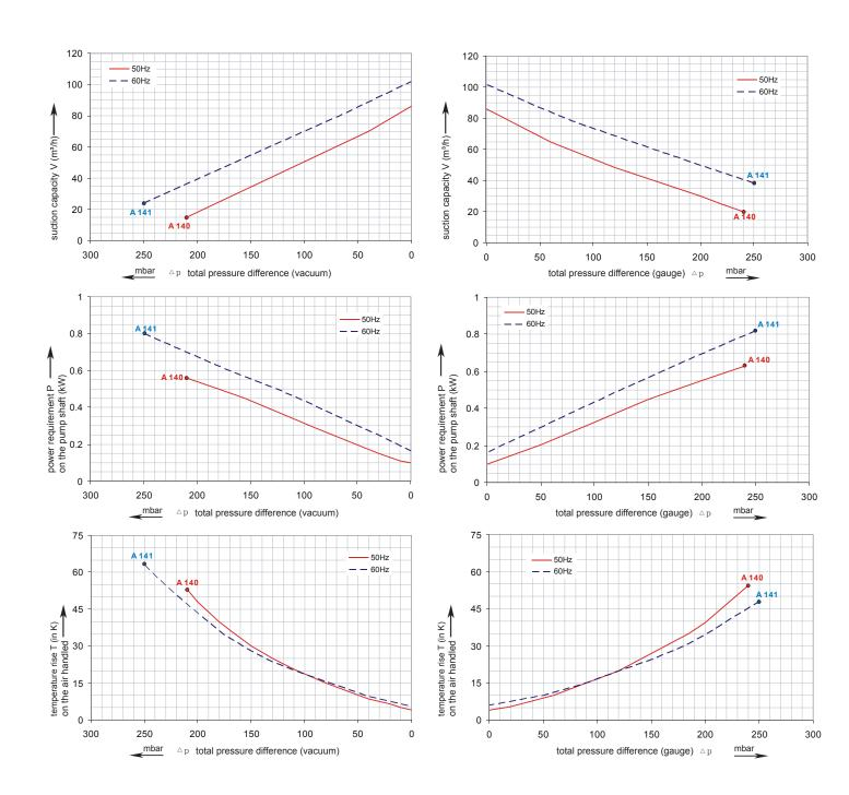
The performance curves are based on air at a temperature of 15  $^{\circ}$ C and an atmospheric pressure of 1013 mbar with a tolerance of +/- 10  $^{\circ}$ C. The total pressure differences are valid for suction and ambient temperatures up to 25  $^{\circ}$ C.
